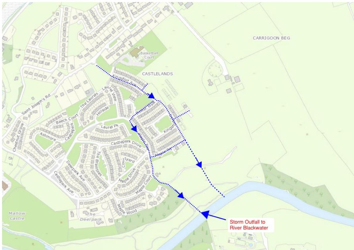
**Figure 2.1 – Stormwater Outfall**
